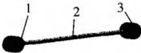
Non-adjustable length tie rod (1.3. Rubber bushing, 2. Steel railing)
